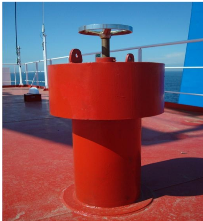
Figure 3.5-16 Type B rotary mushroom-shaped ventilator pipe allowed for areas described in paragraph 5.2.1
